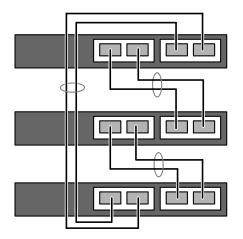
1-port interface modules do not support port aggregation in the IRF. When 1-port interface modules are connected for an IRF, the port of MOD 1 can only be connected to the port on MOD 2, as shown by callout 1 in Figure 3-29; when a 1-port interface module is connected to a 2-port interface module for an IRF, the port of MOD 1 can only be connected to the right port of the 2-port interface module, as shown by callout 2 in Figure 3-29.
